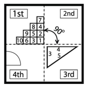
Note: Most rooms are not dead square, so it will be necessary to adjust the lines to get them at 90 degrees. You can do this by marking out a triangle with sides of 4 units x 3 units x 5 units.
